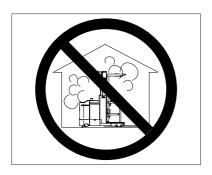
Don't perform battery charging service in the room without adequate ventilation.
