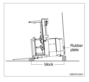
▲ Before performing any maintenance work, check the truck for stable condition on the blocking.
