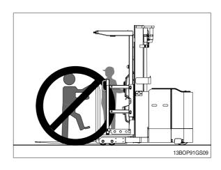
▲ Never try to repair the mast, carriage, chain, or attachment yourself. Always get a trained mechanic.
